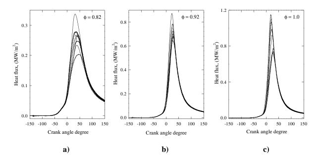
Figure 3- Heat flux variation per crank angle degree: a)  $\phi = 0.82$ , b)  $\phi = 0.92$ , c)  $\phi = 1.0$
