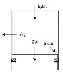
Figure 1- Open system boundary.
