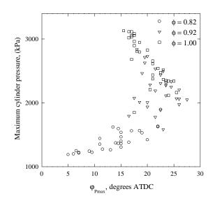
Figure 5- Maximum cylinder pressure as a function of its crank-angle degree.
